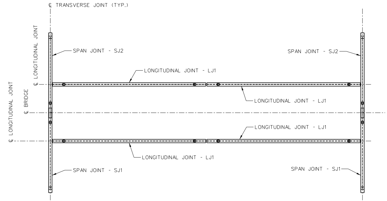
SPAN COVER PLATE LAYOUT SCALE: 3/8" = 1'-0" 30' (NOMINAL) SPAN SHOWN.
